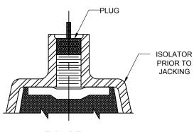
FIGURE 1 PLUG APPLICATION ILLUSTRATION SHIPPED LOOSE
